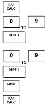
Start the calculator operation. An arrow is shown on the display above the word "CALC"
